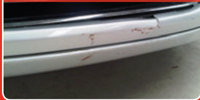
Bumper scratches and crack
