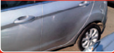
Poor repair: repainted panel does not match
